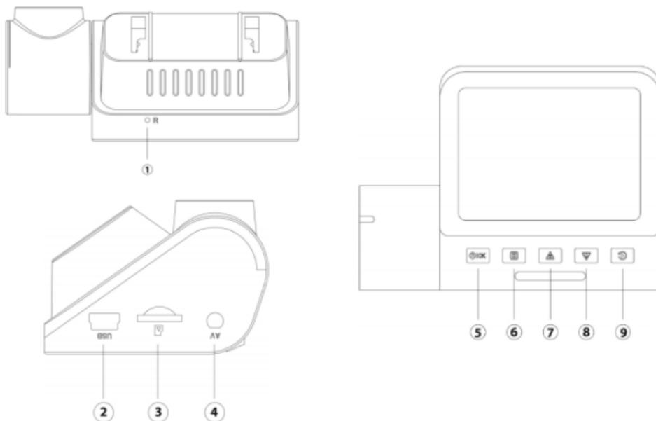
1. Reset port - insert the pin to restart the dashcam
